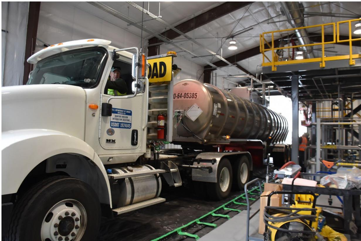
A tanker unloads at a backup load-in station at the Effluent Treatment Facility on the Hanford Site. Driver Nick Bass delivers 6,200 gallons of leachate collected from a mixed-waste burial trench.
