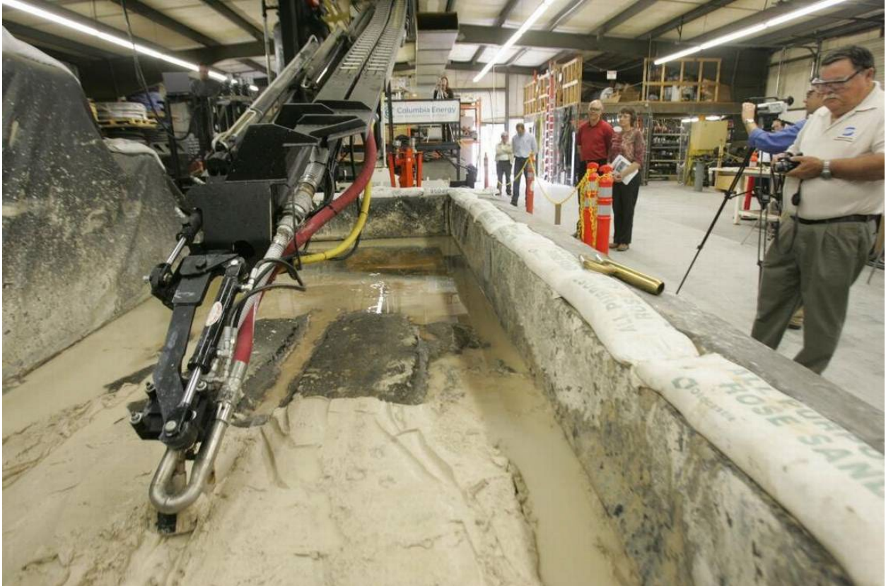
The vacuum Mobile Arm Retrieval System is shown during testing with a waste simulant before the robotic arm vacuum system was used to empty some of the waste from Hanford's Tank C-105. File Tri-City Herald
