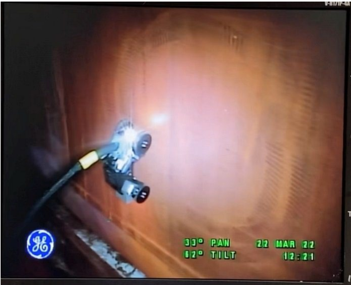
A mini crawler, developed by Florida International University students and faculty, moves along the outside of the inner tank shell on a double-shell waste-storage tank at the Hanford Site.
