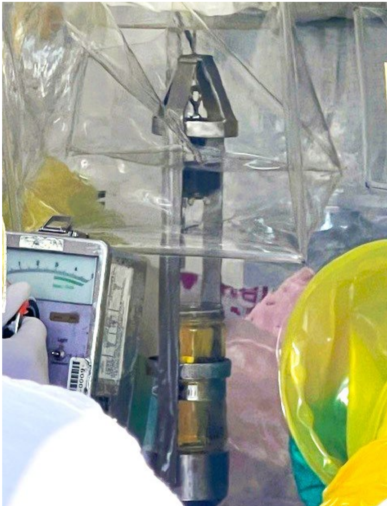
The 222-S Laboratory, operated by Hanford Site contractor Navarro-ATL, tests liquid waste from the underground storage tank that will feed it to Hanford's Waste Treatment and Immobilization Plant.
