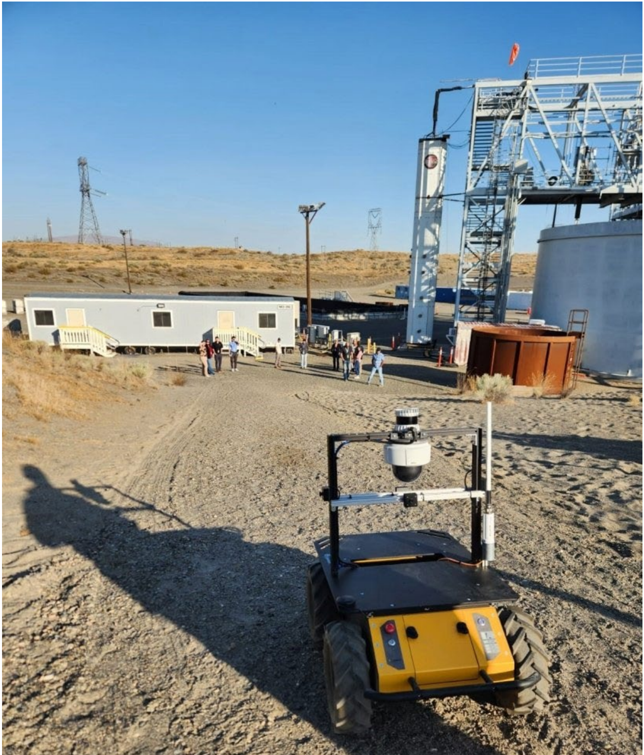
A robot used on the Hanford Site is remotely controlled and can be equipped to complete various tasks in conditions that might be hazardous for humans.
