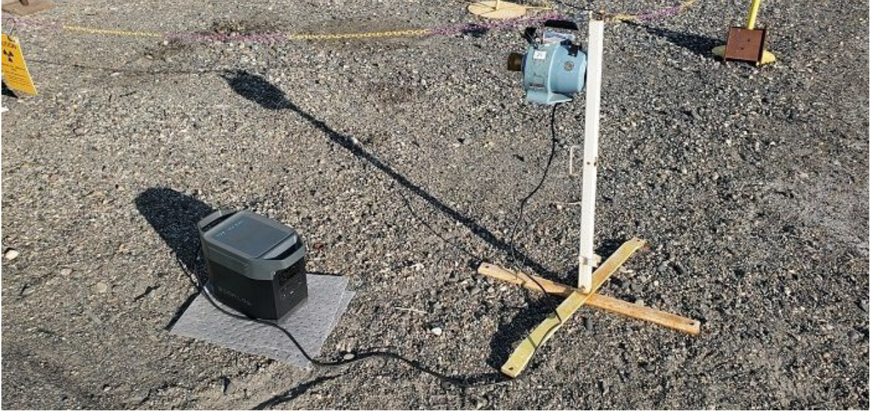
New, zero-emission electric generators being used in the Hanford Site tank farms are quieter than their gas-powered counterparts, require less upkeep and eliminate potential exposure to exhaust fumes.
